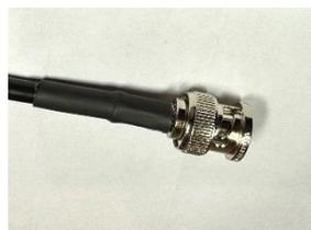
If you have a multi-meter, check the cable end to end now for continuity / no shorts then finish the plug off with suitable heat-shrink tubing.
