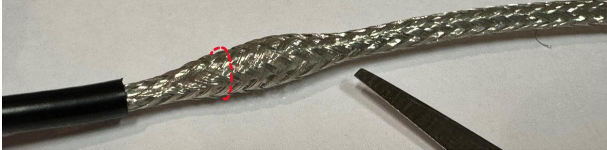
Bring the pipe up to the level of the end of the black outer cable insulation and wrap the remaining braid over the edge of the pipe keeping it level with the start of the (now exposed) centre insulation
