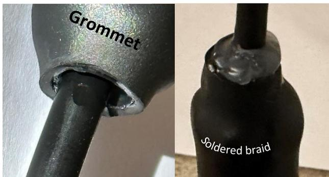
Insert hot melt glue into the upper opening with glue gun and/or re melt with the heat gun.
