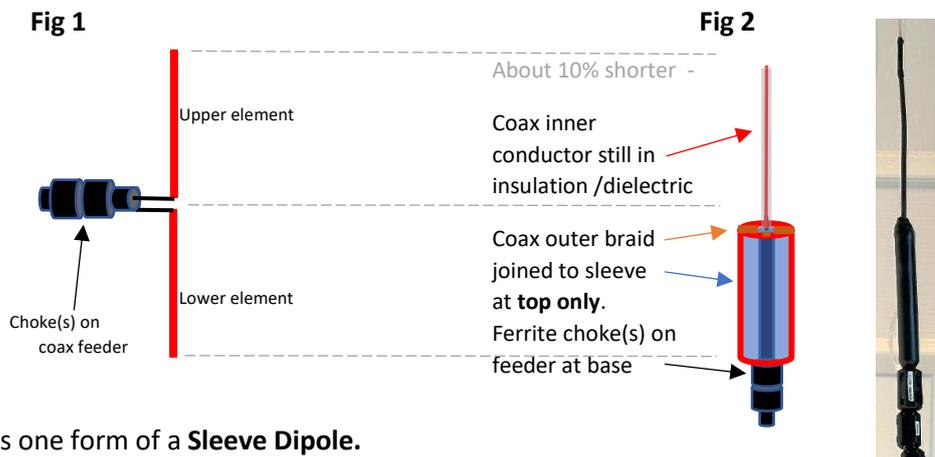
**Fig 2** is one form of a **Sleeve Dipole**.
