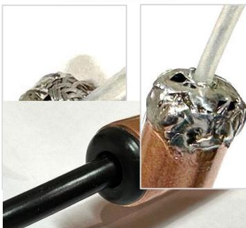
At the bottom end, push one grommet up into the middle of the pipe. Drip down superglue between the grommet and inner pipe. Then insert the second grommet into the bottom end and apply superglue to both the grommet/pipe and cable/grommet areas (don't block them completely at this stage). Leave it all to set.
