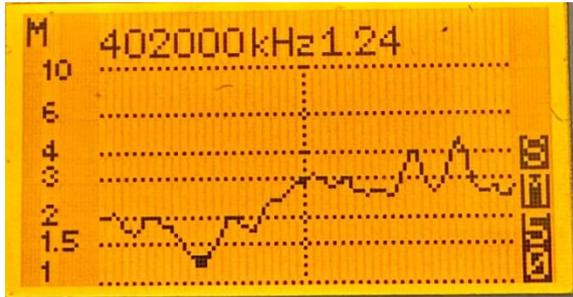
Trim 0.5 to 1mm off the coax centre length each time before replacing heatshrink and re-measuring
